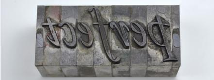
Metal type with *kerns* makes all the difference in the spacing between certain character pairs, such as 'rf', 'fe', and 'ct' (lower). Photographs courtesy of Lead Graffiti.
